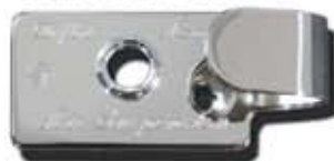
PA-02AS S/S - Switch Guard - Air Suspension
